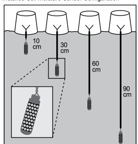
Installed Soil Moisture Sensor Configuration
